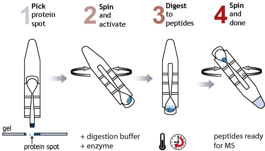
**Fig. 2 Illustration of the picking process**
